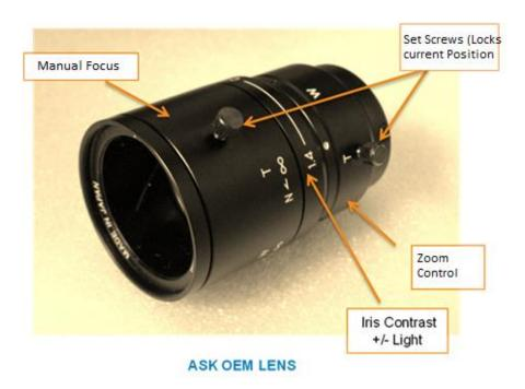
The OEM lens is a C-Mount type. It has a variable zoom from 4mm – 12mm. The lens also has the option to open or close the iris. This will allow the person setting up the camera and lens more adjustability when determining the correct brightness level. The manual focus control at the front of the camera allows for fine adjustments to be made to make the image as clear and focused as possible. Color and Polarized filters are available for purchase through A.S.K. Technologies.
