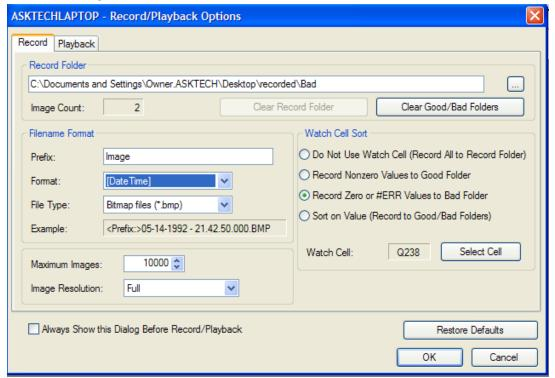
Once you have confirmed that the Record Setup Screen above matches yours, you need to save the job. Select "File" from the top of the screen and choose, "Save Job". Also save the layout so that the record button will stay where you added it. To do this select "System" from the top of the screen and choose, "Save Layout". \*Record button needs to be pressed only once at system startup, but needs to be done every time the system is shut down or turned off.
