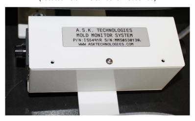
The remote control unit houses the main operator control components of the mold monitor system. This includes the power switch, timer, reset button, and a 6 pin plug for the cameras power/communication cable. The power switch and 6 pin pug are located on the back of the remote control unit while the time is on the left and the reset button is on the right.
